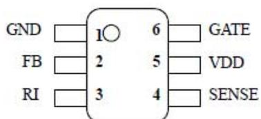
Figure 1. Pin Assignment of EST2263 for SOT23-6
