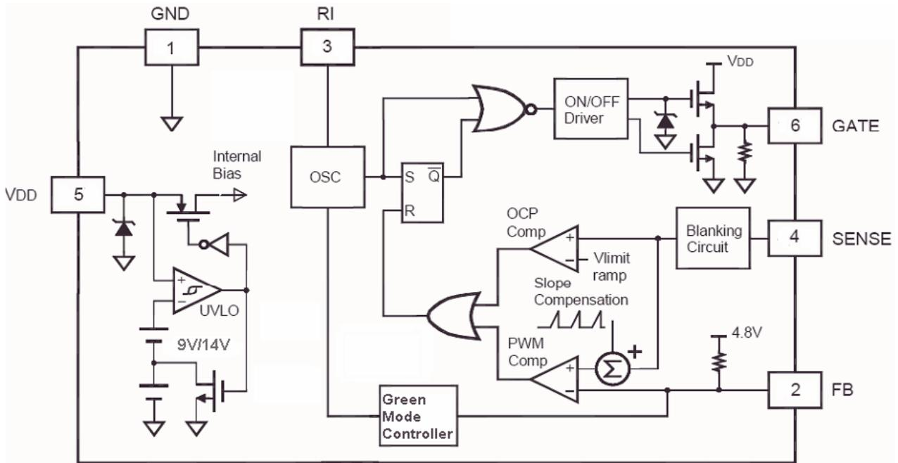
Figure 4. Block Diagram of EST2263
